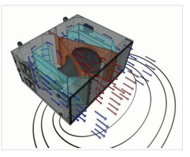
hybrid combination between a short transmission line and an over-damped reflex load. Moreover, the maximization of the mutual coupling between the drivers increase the fastness of the transient response while maximizing the overall energy efficiency as well.
